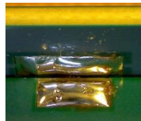
Solder melted, leaving gap, but excess
